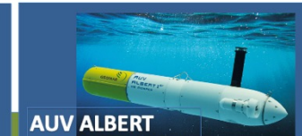
AUV ALBERT (4 kn / 200 m / 50 kg)
